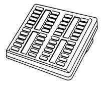
The indicators turn on one at a time in sequence, beginning at the lower right corner of the module. The indicators then turn off. After all the indicators turn off, the CAP module is initialised and ready to use.
