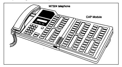
By pressing a ringing line button on your CAP module and lifting the handset, you can answer a call made from outside your Enterprise Edge system. Pressing the appropriate programmed memory button allows you to automatically dial an internal or external number, or use a feature.
